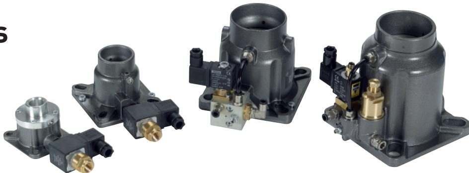
**APPLICATION:** Installed on the compressor inlet to control its capacity. At start-up, the valve remains open till the minimum suction pressure closes the valve. During normal operation, the valve opens and closes in response to a signal that meets the air demand.
